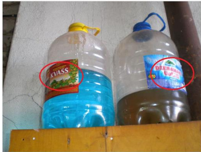
Chemicals stored in reused containers that are not labelled with the name of the chemical
