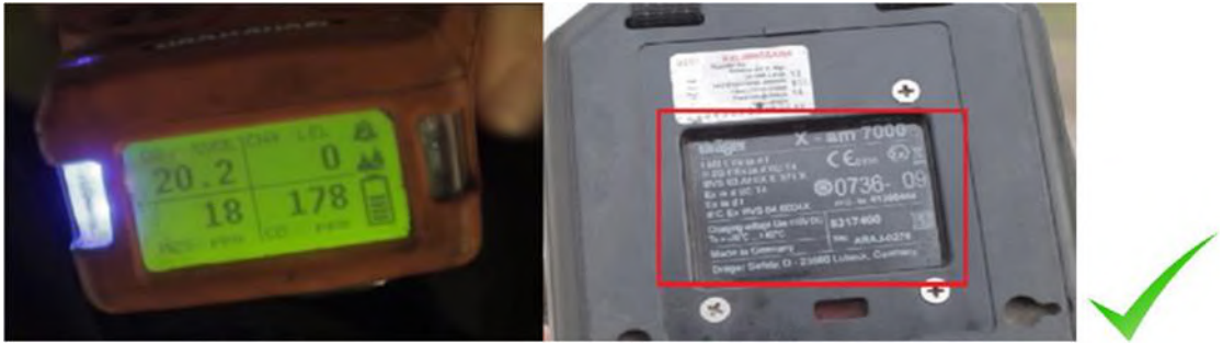
Air quality analyser suited for working in an explosive environment (0, 1, 2) and at VTL
