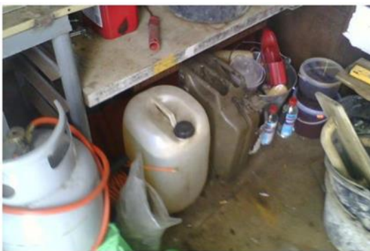
Cans full of fuel are kept with combustible materials
