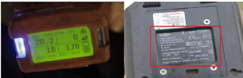
Air quality analyser suited for working in an explosive environment (0, 1, 2) and at VTL
